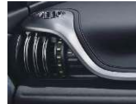
Dumbbell-style Air Conditioning Vents
